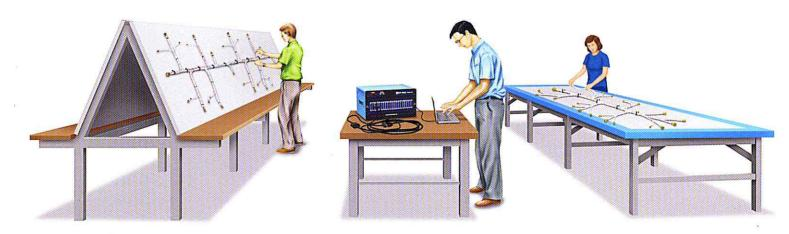
The Model 2115 fits into lean environments. The system's small footprint allows locating the tester in the fabrication area or moving it throughout the production facility.
