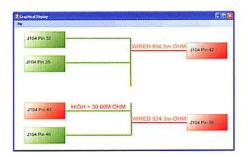
The continuity probe is used to verify connections to loose conductors. Both visual and audible indicators identify passing tests. With the automatic advance, the probe can be used to simply step through the loose wires.
